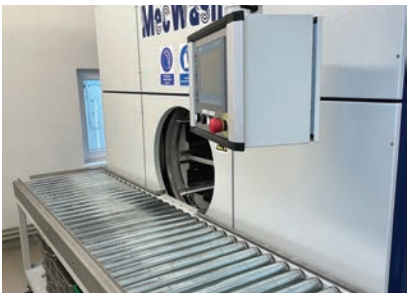
Ultrasonic parts washing capable of meeting cleanliness requirements.
