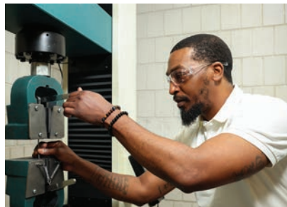
Tensile and wire testing ensure raw material standards.
