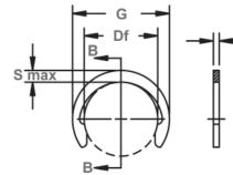
Free Diameter & Ring Measurements With Section B-B
