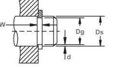
Shaft Diameter & Groove Dimensions
