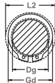
Clearance Diameter & Gaging Diameter Released in Groove
