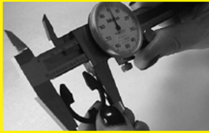
Caliper measuring outside diameter of ring
