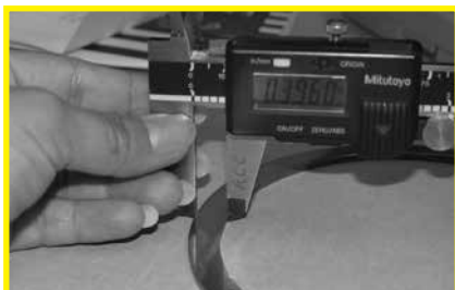
Measuring S max on an HO Retaining Ring.
