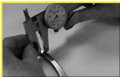
Measuring S min on an HO Retaining Ring.
