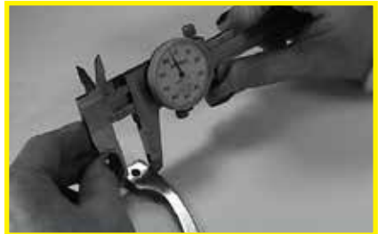
Measuring lug height (H) on an HO Retaining Ring.
