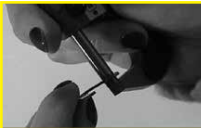
Micrometer measuring thickness (T) of PO (Poodle) ring.
