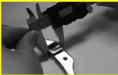
Measuring lug height (H) on an SH Retaining Ring.
