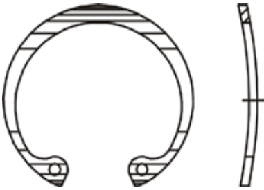
BHO- Bowed HO Retaining Ring.
