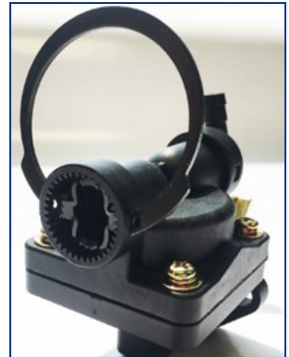
*The inverted lugs of the HOI ring are expanded and installed on two tabs of the opening of this fuel pump repair kit*
