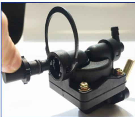
*The fitting for the fuel hoses can now be inserted as shown above*
