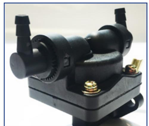
*Once the ring is removed, the fittings are locked in place and ready to be connected to the fuel hoses.*
