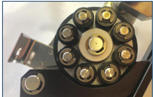
The eight rollers are held in place by E retaining rings; an E ring also retains the entire wheel the rollers are attached to.
