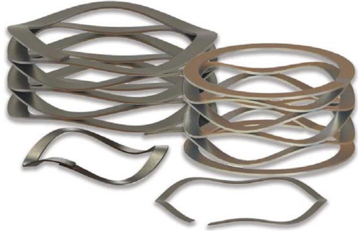
Single turn wave springs are ideal for short deflection applications with low to medium forces. They are offered in a number of waves and material thicknesses and designed for a wide range of bore and rod diameters. Available in gap and overlap designs. Multi turn wave springs are available in a wide variety of loads, deflections and diameters. They are ideal for medium and heavy duty applications and have high thrust load capacity. Available with plain or shim ends.
