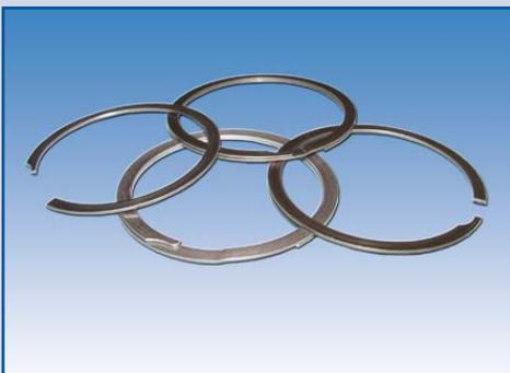
Spiral rings are axially installed into machined grooves in housings/bores or on shafts to retain assemblies. They provide 360° contact with the groove and offer more clearance than a tapered section ring.
