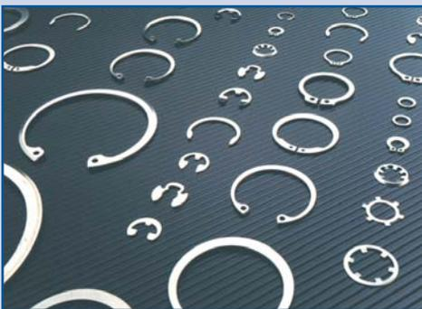
Axially assembled retaining rings are designed for axial installation into machined grooves. These rings are either internal for installation in housings and bores, or external for assembly on shafts. Once installed, they provide a protrusion or "shoulder" for retaining parts.
